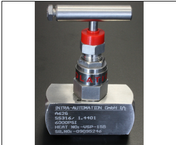
Fig. 21: Needle valve 1/2" NPT, PN400 (5801 psi); 1.4401 (316SS) (A62)
